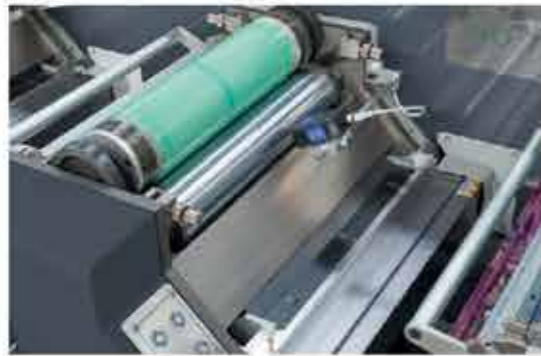
Flexo Print Unit with Gear Cylinder (Single Servo)
