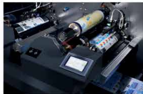
Sleeve system with 3 servos
