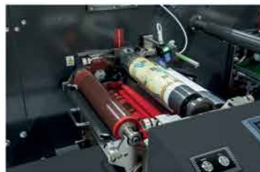
Gear Cylinder System with 2 servos (Flower Style)
