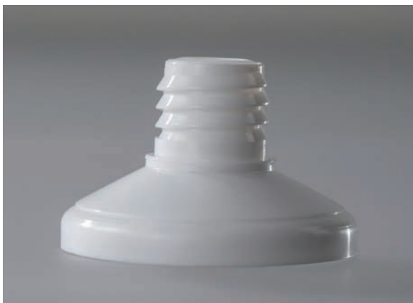
This HDPE tube collar with a total shot weight of 81.6g is produced on an all-electric e-mac 740/280 injection moulding machine, using a 48-cavity mould.
