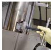
**Melt filters** for continuous removal of solid contaminants are available. The optional backflushing function reduces costs for filter screens and operator intervention. In case of higher contamination, a power backflushing or continuous melt filter is recommended.
