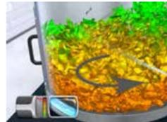
Large SMART feeder for a wide range of input materials. Enlarged operation window due to water cooled bottom.
