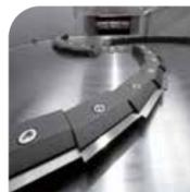
**The SMART feeder** optimally prepares the input material and feeds it into the extruder by centrifugal force. **The dynamic automation package** regulates the ideal operation point. Automatic speed adjustment of rotating disc and positioning of load-controlled intake slider leads to increased output. Higher levels of humidity can be processed.
