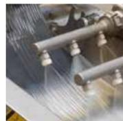
**The pelletising system** is chosen depending on vpolymer type and preferred pellet shape. In case of automatic strand pelletising, broken strands are automatically inserted into the strand pelletiser without operator interference. Alternatively, manual strand, water ring, or underwater pelletising are available.
