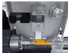
Optimally prepared material is continuously fed into the extruder by centrifugal force.
